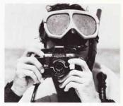
24. Take the picture. Look through the view-finder, and depress the shutter release button halfway. If the LED doesn't blink, depress the button all the way to take the picture. The shutter speed automatically selected is between approx. 1/30 sec. and 1/1000 sec. If the LED does blink, readjust the aperture until it stops blinking.
