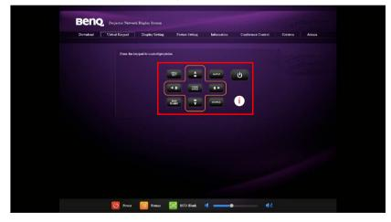
These buttons function the same as the ones on the remote control. See "Remote Control" on page 14 for details.
