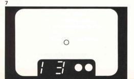
readjust the Eyepiece Adjustment Lock Ring to a midway point so that both the digital display and 1° spot appear reasonably sharp.
