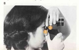
until it stops. When someone else is to use the spotmeter, rotate the Eyepiece Adjustment Lock Ring counterclockwise to loosen eyepiece, readjust eyepiece, and lock it into place once again. Illust. 10, Align the ASA No. of the film being used with the green ASA Index (⑦, illust. 10) by rotating the ASA/Shutter Speed Dial (⑥) which is close to the front of the lens ⑤). The figures of the ASA Scale also appear in green.
