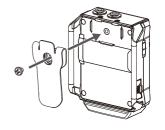
Connect the lavalier mic to the MIC/LINE IN jack, and tighten the screw lock.
